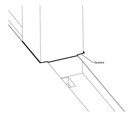
**Install Downspout**Place the downspout over the gutter outlet and secure with screws to the column. Install hole plugs.
