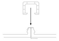
Repeat the process of placing a canopy panel, snapping a batten into place, and installing mounting clips along the length of the canopy panel until all canopy panels are installed.
